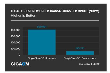
Figure 6. TPC-C Highest New Order Transactions per Minute (NOPM) (Higher is Better)
