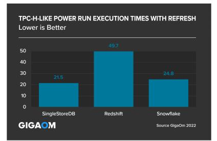
Figure 3. TPC-H-Like Power Run Execution Times with Refresh (Lower is Better)
