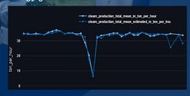
Detect drift of turbine power production in relation to incoming steam tonnage and steam extraction for the DHN
